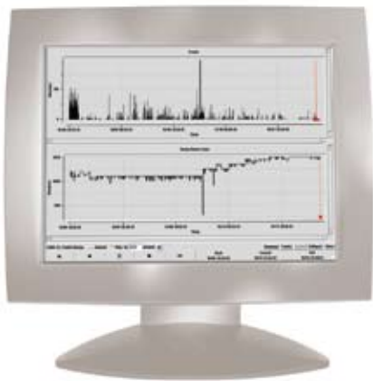
Route Explorer provides the ability to review and replay routing events. This view shows a histogram, which enables easy identification of when significant events took place.
